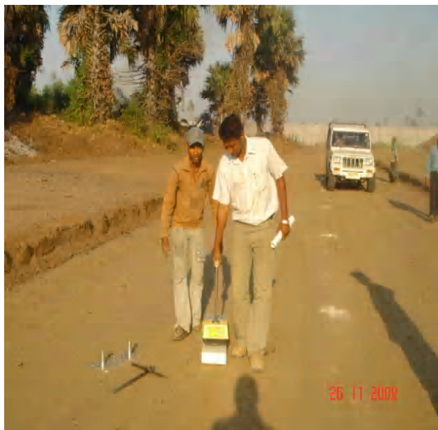
Fig. 4: Photo Plate Showing Testing with NDG
